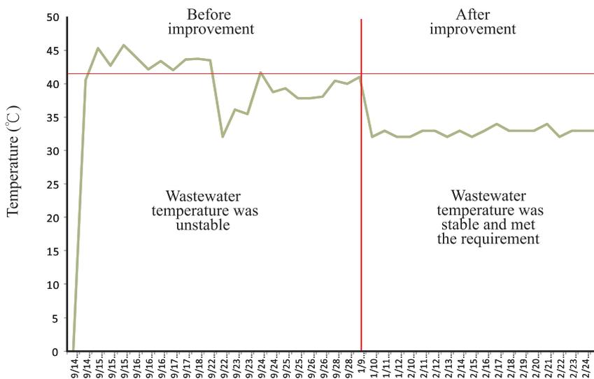
**Fig.7.** The trend of wastewater temperature as a function of time.
